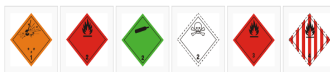
1-Explosives 2.1-Flammable gases 2.2-Non-toxic and non-flammable gases 2.3-Poison gases 3-Flammable liquids 4.1-Flammable solids
